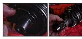
The needle bearings should slide easily with no obstructions. And don't forget the circlips as you go.
